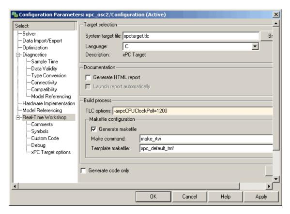
If you want to execute the target application in interrupt mode again, either remove the option or assign a CPU clock rate of 0 to the option:
