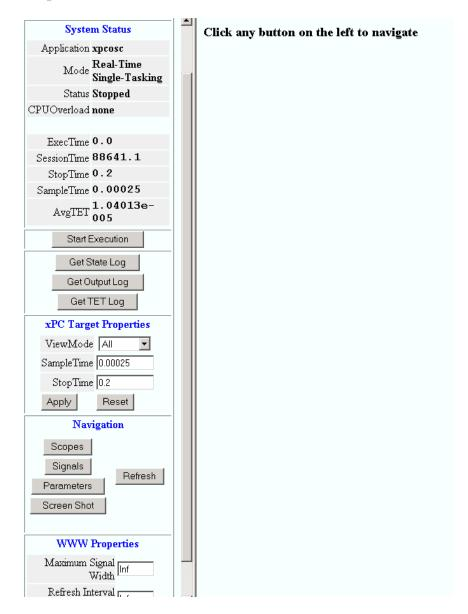
After you connect a Web browser to the target PC, you can use the **Main** pane to control the target application:
